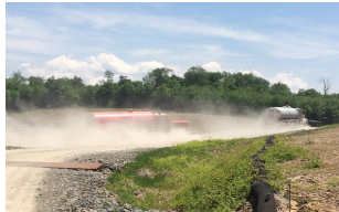
Dust from Truck Traffic at Well Pad.
